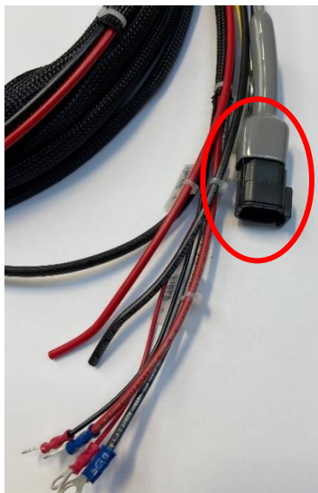
Yanmar Connection on the Controller Loom
